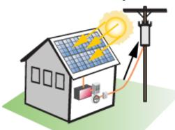
In the middle of the day when the solar system produces more energy than is needed onsite, the extra power is exported to the grid and the meter runs backward, building up a credit with the utility.
