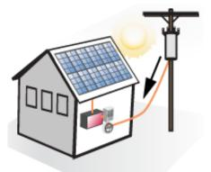
In the morning hours when the solar system produces less electricity than needed, the customer will pull electricity from the grid.
